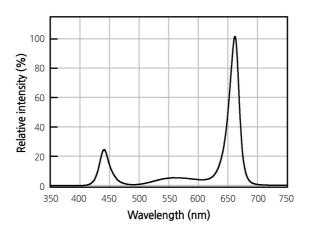
Fig. 1. Relative spectral distribution for LEDs (R:W:B = 7:2:1) used in this study. Spectral scans were recorded at 25 cm from the lighting sources and at five points (center and four corners of each tray of pots) with a spectroradiometer.
